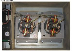
4. There are four motor brushes; two on each motor. They are outlined in red in the above picture. Circled in red are the screws that hole the motors in place. Turn each of these screws approximately 2 rotations. This should be enough to loosen the brushes enough so you can remove them by lifting and sliding them out:
