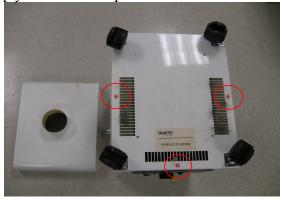
3. Notice three screws are circled in red. Remove these screws and pull the bottom panel off of the machine, wheels and all. Your unit may have additional screws in the corners as well. Now you should be able to see the backs of the two motors that run the fans. It should look like this:
