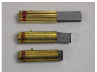
6. If any of the brushes need replaced, it is best to replace all four at the same time. Slide in the new brushes in the proper orientation and screw them down securely. Reattach the bottom panel, and screw it in. Flip the unit right-side up, insert the filters, and reattach the top. Reconnect the unit to the laser machine.
